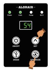
Press and hold 'SET' and 'GPP MODE' together for 3-5 seconds.
