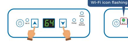
Press and hold 'UP' and 'DOWN' together for 3-5 seconds.
