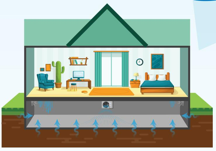
Fan-powered crawl space ventilation quickly reduces moisture and humidity which helps in protecting both the home and the occupant. This crawl space fan increases air circulation to fight condensation and ventilates excess moisture which can be the cause of mold, mildew and wood rot. The constant operation of this unit helps vent radon, treated wood off-gassing and odors that might otherwise migrate into the living spaces of the home.
