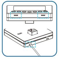
Gently insert a flathead screwdriver or a similar tool into the two slots provided. Carefully pry the unit open by applying gentle pressure.
