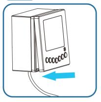
Attach the control board to the switch box as shown above.
