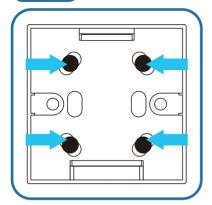
Position the switch box in the desired location and use the four screws provided to secure in place.
