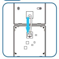
Insert the CAT-5 cable into the corresponding port on the control board. Listen for a distinctive clicking sound, which indicates a successful connection.
