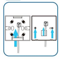
Thread the wire through the designated opening in the cover shell. Next, align and secure the switch box using two screws.
