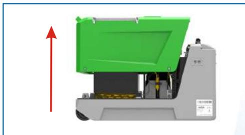
1. During the dis-assembly of unit, the front board can be take away directly without the interference of any power lines.
