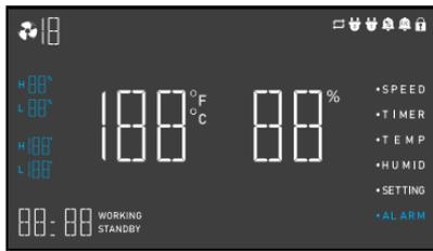
Press the menu key once again to move you to the low-temperature option. You will then scroll up or down to enable you to choose the low-temperature trigger. If the values of the humidity or temperature fall below the trigger point, the fan ignores the settings. Thus, it triggers the alarm. Turning to the 10th gear
