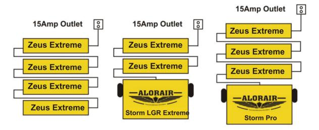
**NOTE:** The Zeus Extreme plugs into standard 115 VAC electrical outlets.
